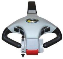
The degree of rotation determines the speed of movement, so the farther you press the wheel in either direction, the faster the stacker will travel, up to a maximum speed of ~3mph when loaded ~2.6mph when unloaded Simply by releasing the movement capacity. control, the stacker will decelerate to a complete stop.
